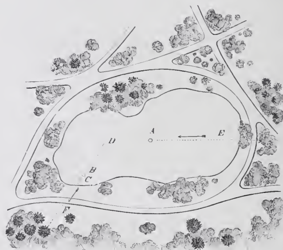
Fig. 56.—CITY PARK POND, HARTFORD, CONN. A. Fountain; B. Outlet; C. Overflow; D. Outlet Sink; E. Supply Pipe; F. Outlet Overflow Pipes.
